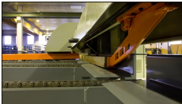
Stringer pusher with servo-motor
